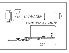
steam space to the condensate outlet or a internal bleed incorporated into the steam trap design.
