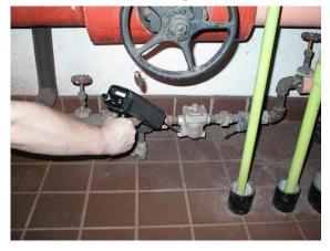
and is used as a predictive tool for steam trap monitoring. Ultrasonic testing permits the testing person to hear the internal operation of the steam trap; so the effectiveness of the steam trap operation can be determined.
