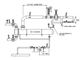
condensate passing through the steam control valve will cause premature failure of the control valve The buildup of condensate can simple be eliminated by installing a drip leg prior to the valve. This allows the condensate to fall into the drip pocket and be evacuated with the assistance of a steam trap.
